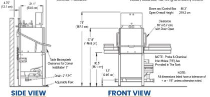
\*Requires external hot water source that will provide at least 47 gallons of 180 degree water an hour Effective 2/2023
